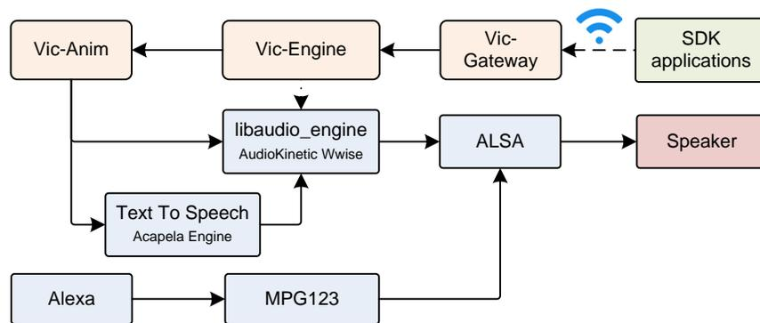
**Figure 107:** The audio output architecture
