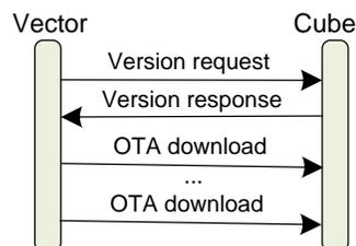
**Figure 60:** Sequence for sending the Cube firmware
