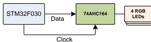
**Figure 19:** SPI-like interface to the 74AHC164 and RGB LEDs
