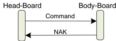
**Figure 52:** Body-board NAK a CRC-error or bad command
