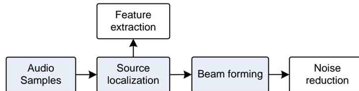
**Figure 68:** Typical spatial audio processing flow
