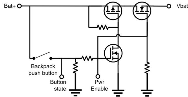
**Figure 11:** A representative battery connect switch
