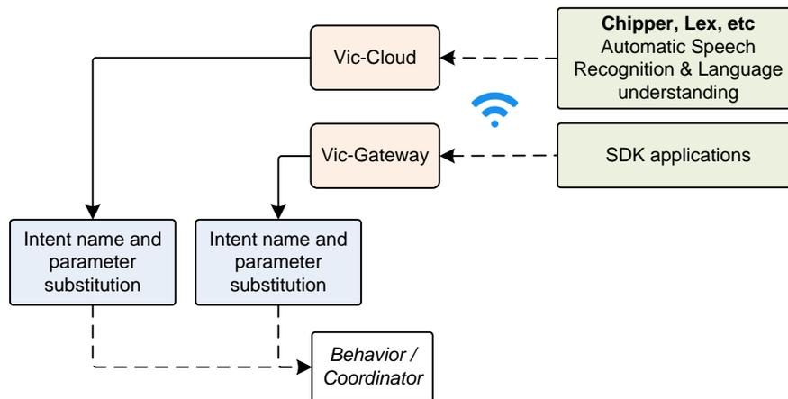
Figure 74: The filtering of intents
