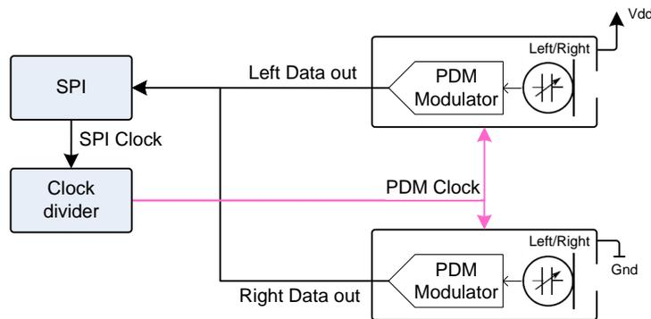
**Figure 16:** Sampling two microphones with a single SPI master (adapted from ST Microelectronics)
