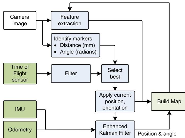
**Figure 91:** A typical localization and mapping functional block diagram
