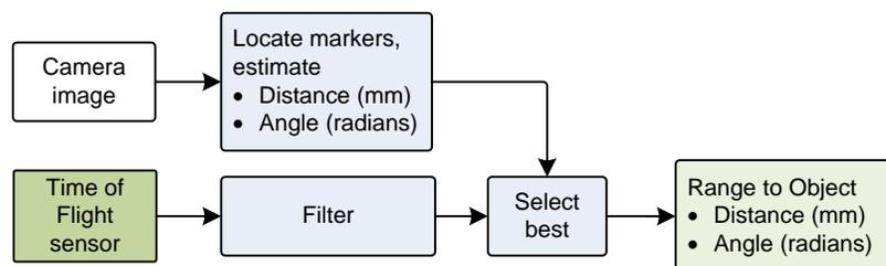
**Figure 87:** A typical localization and mapping functional block diagram
