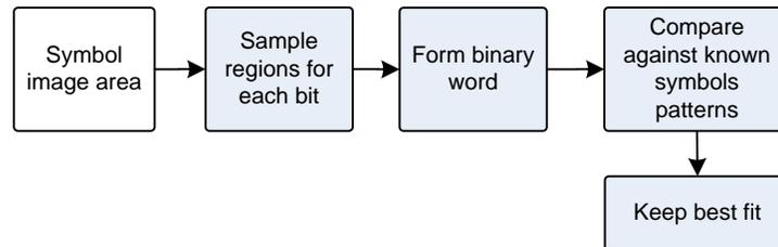
**Figure 81:** Decoding the symbol
