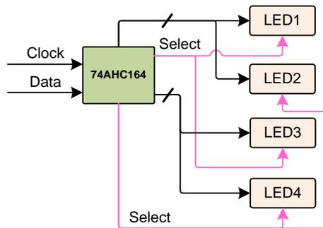
**Figure 8:** Possible light topology on backpack board
