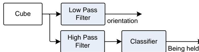
**Figure 92:** Sensing motion events
