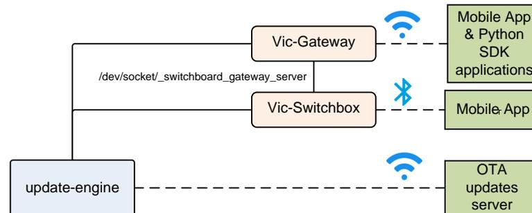
**Figure 131:** The architecture for updating Vector's software
