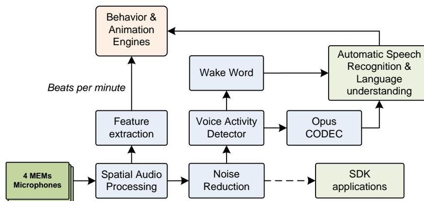
**Figure 64:** The audio input functional block diagram
