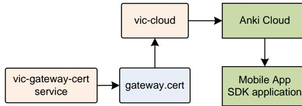
**Figure 47:** The certificate flow from the robot to the mobile application
