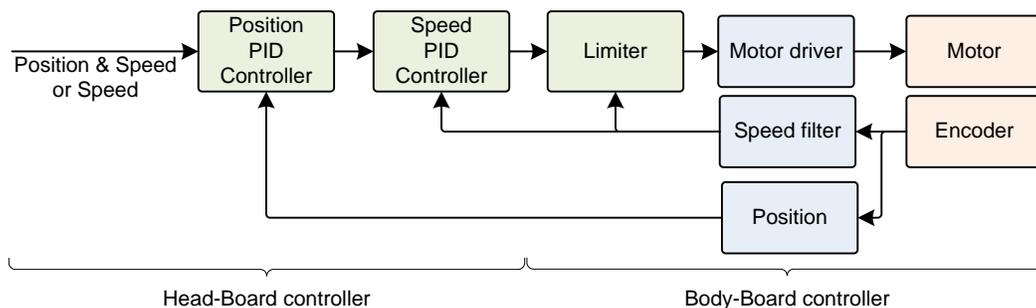
**Figure 117:** A typical motor control loops, as they might appear in Vector
