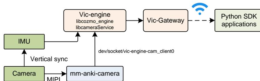
**Figure 32:** The camera architecture
