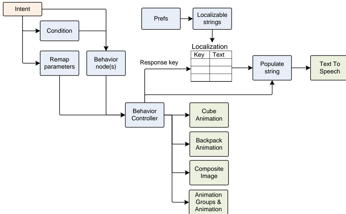
**Figure 123:** The behavior controller links together multiple intents, and responses
