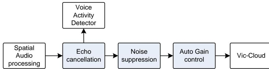
**Figure 69:** Typical audio noise reduction flow
