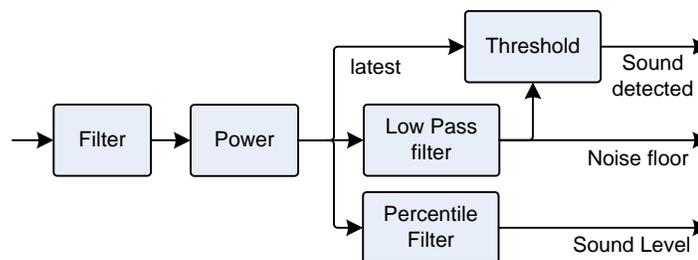
**Figure 70:** Sound and noise level estimator, and activity detector
