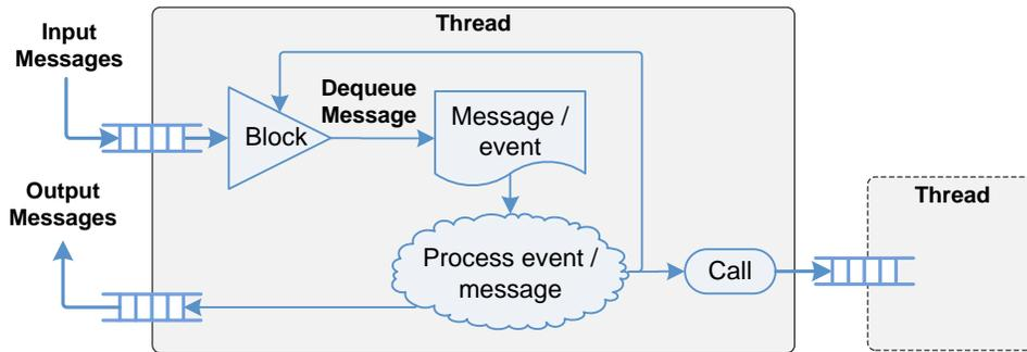
**Figure 27:** Basic communication thread structure
