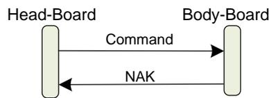
**Figure 52:** Body-board NAK a CRC-error or bad command
