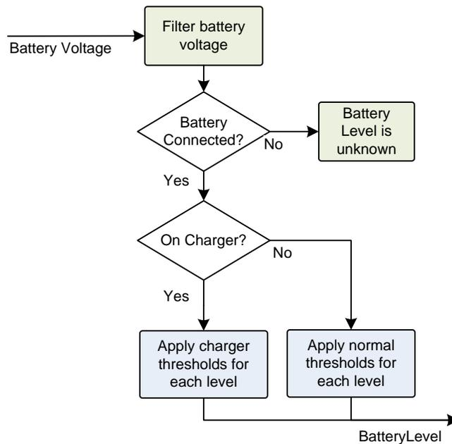
**Figure 34:** The battery level classification tree
