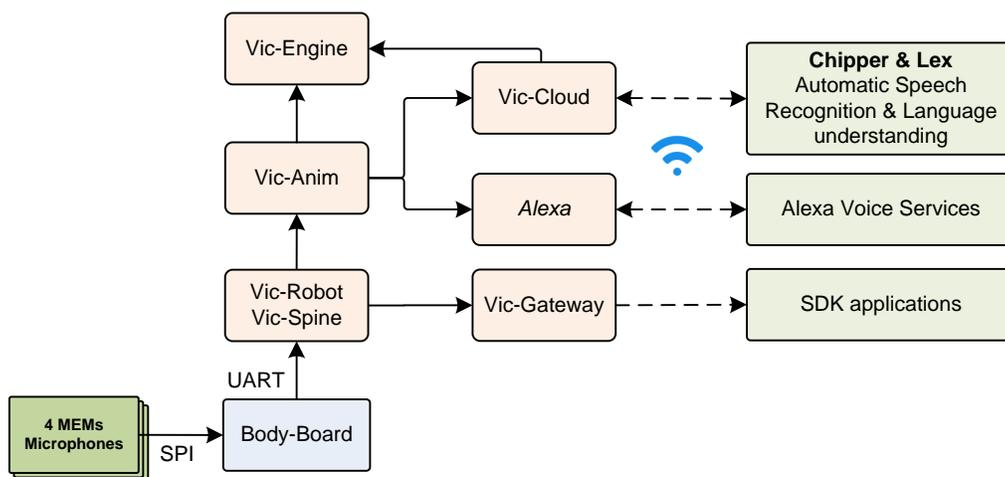
**Figure 65:** The audio input architecture
