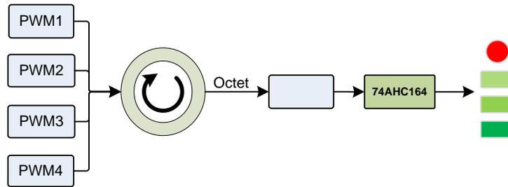
**Figure 40:** The firmware driving of the LEDs
