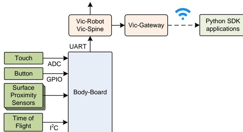
**Figure 37:** The touch and button input architecture
