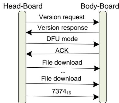
**Figure 53:** Sequence for updating the body-board
