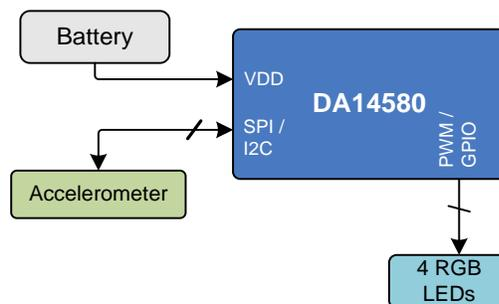
**Figure 24:** Block diagram of the Cube's electronics
