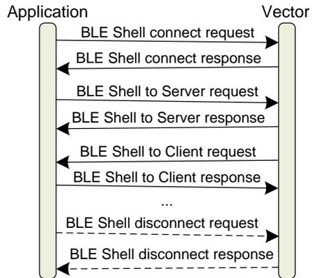
**Figure 59:** Sequence for communication with a command shell on Vector
