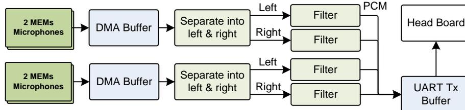
**Figure 66:** Sampling the microphones and converting to PCM format
