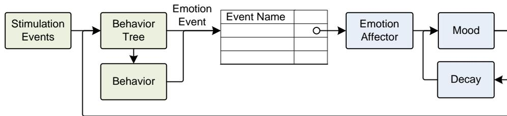
**Figure 126:** Mapping an emotion event to how it impacts the emotion model
