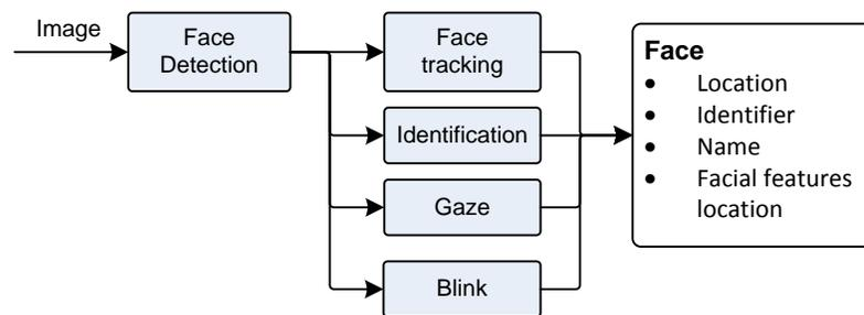
**Figure 82:** The face detection and recognition processes
