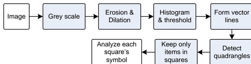
**Figure 80:** Preparing image for scanning for symbols
