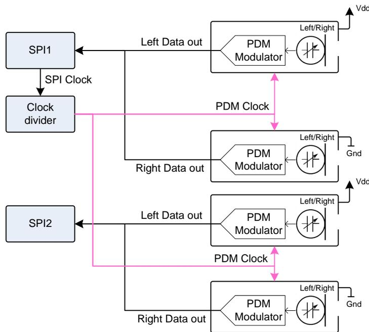
**Figure 18:** Sampling four microphones with two SPI masters (adapted from ST Microelectronics)
