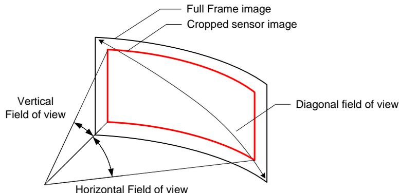
Vector’s calibration uses focal length instead of field of view. The two values are related:
