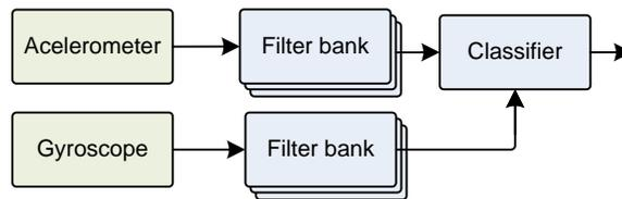
**Figure 43:** Classify movement by filtering the accelerometer and gyroscope signals
