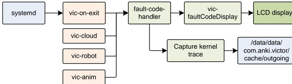
Figure 136: The fault-code-handler process
