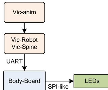
**Figure 39:** The backpack lights output architecture
