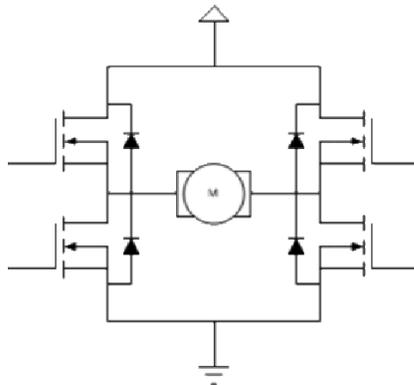
**Figure 20:** Motor driver H-bridge
