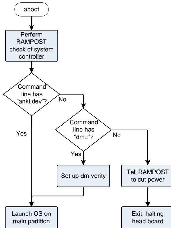
**Figure 33:** The linux boot-partition `init`-script flow
