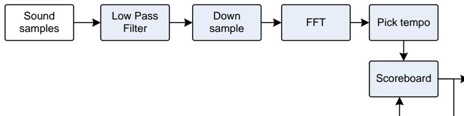
**Figure 72:** Typical tempo measurement
