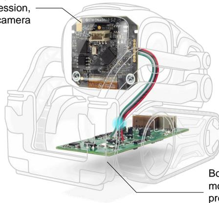
Body board for controlling motors, charging battery; proximity sensors to detect cliff; charging pads
