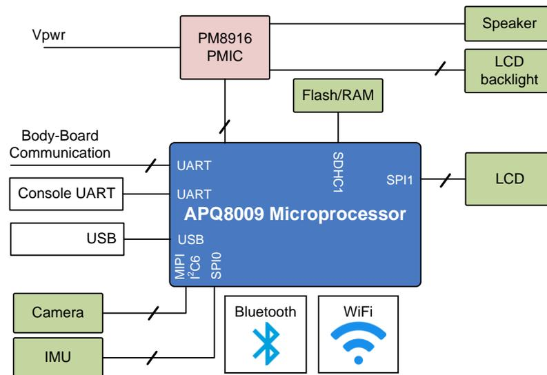
**Figure 6:** Head-board block diagram
