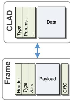
**Figure 50:** Overview of the body-board frames
