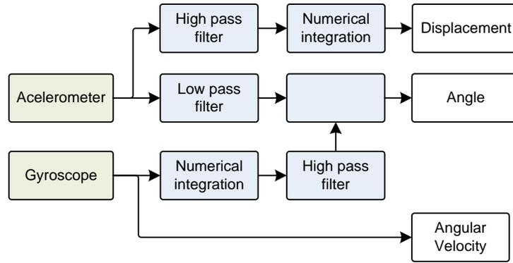
**Figure 42:** Complementary filtering of the accelerometer and gyroscope
