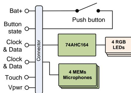
**Figure 7:** Backpack board block diagram
