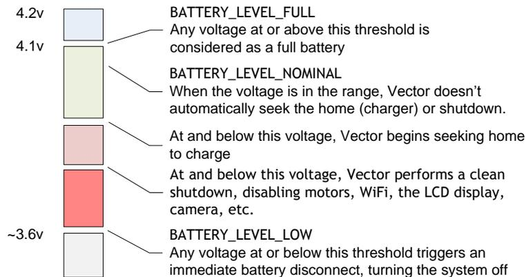
**Figure 35:** The battery thresholds
