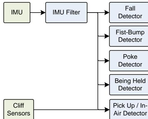
**Figure 41:** Sensing motion events
