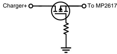
**Figure 12:** A representative PFET based reversed polarity protection
