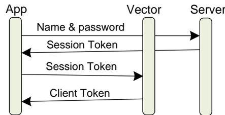
**Figure 48:** Sequence for acquiring a client token
