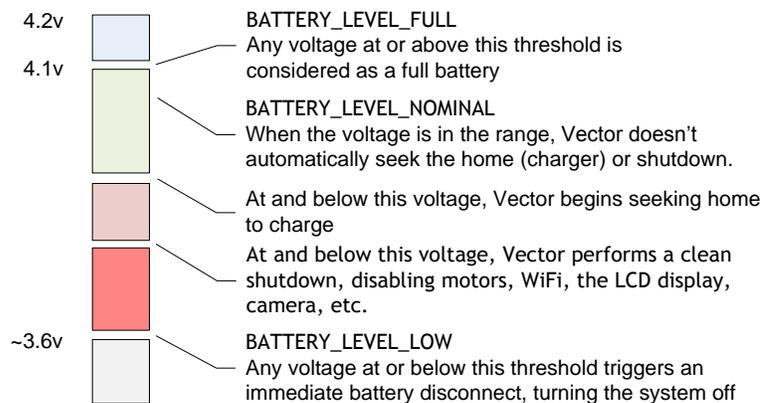
**Figure 35:** The battery thresholds
