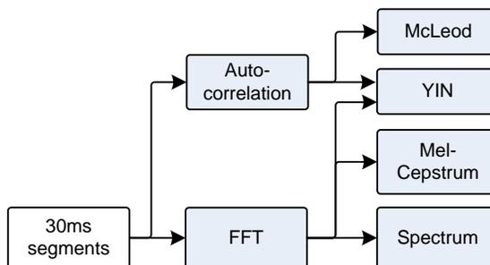
All there are distinctions between these methods, there are far more similarities. They all build on basic techniques like autocorrelation, and *fast-fourier transform* (FFTs). An FFT computes a spectrograph, giving the strength of each frequency. The simplest (or naive) approach is to find the strong frequency and call it a pitch. This approach is easily fooled. A variety of other techniques have been developed to work around this.
