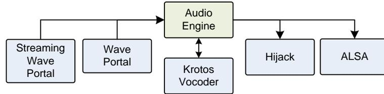
**Figure 108:** Plug-ins in the Wwise audio pipeline
