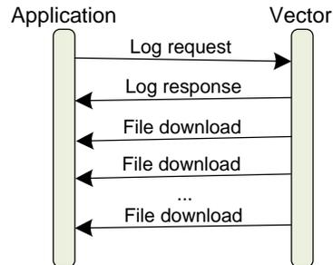
**Figure 58:** Sequence for initiating communication with Vector
