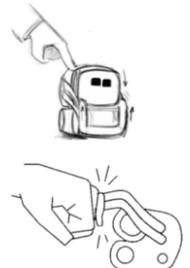
Fall detection is similar. In free-fall, the force measured by the accelerometer gets very small. If Vector is tumbling, there is a lot of angular velocity that is taking Vector off of his driving surface.
