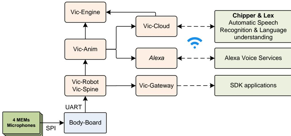
**Figure 65:** The audio input architecture
