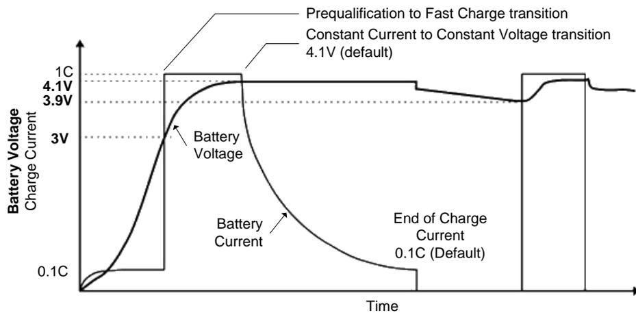
**Figure 13:** Charging profile (adapted from Texas Instruments)
