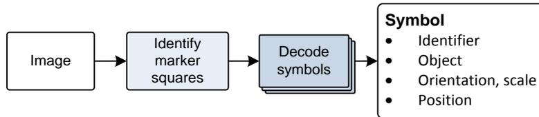
**Figure 78:** The processing of the image for symbols and objects
