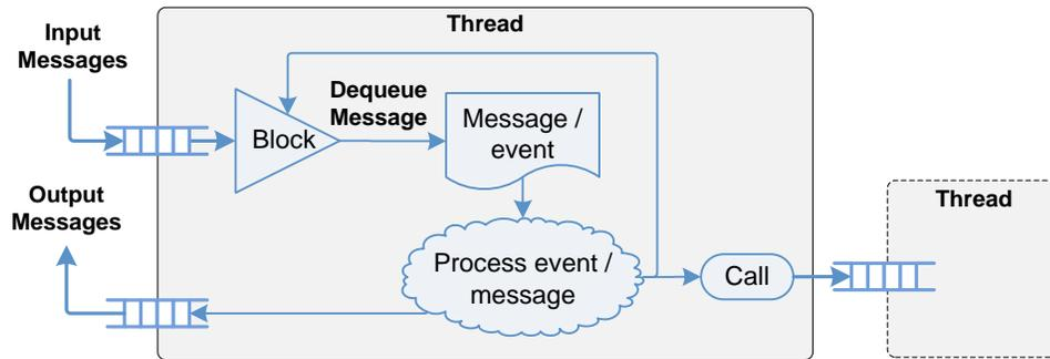
**Figure 27:** Basic communication thread structure
