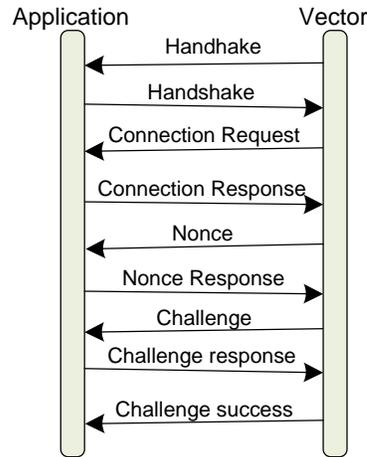
**Figure 56:** Sequence for initiating communication with Vector
