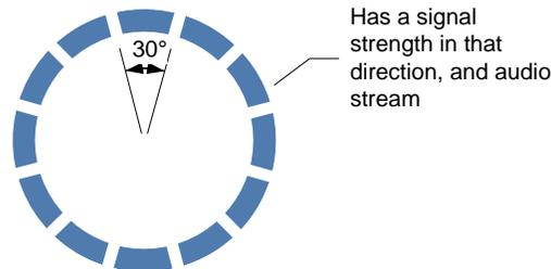
**Figure 67:** The audio can be isolated into one of 12 different directions
