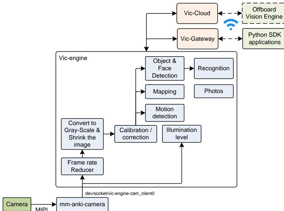
**Figure 75:** The camera architecture
