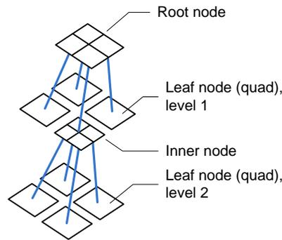
**Figure 86:** Structure of a quad-tree
