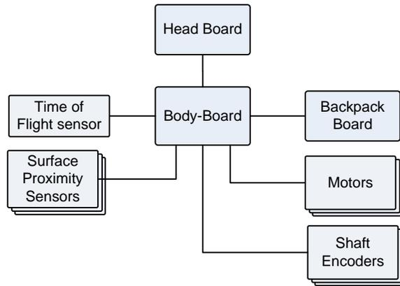
**Figure 3:** Circuit board topology
