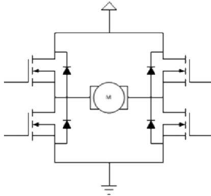
**Figure 20:** Motor driver H-bridge
