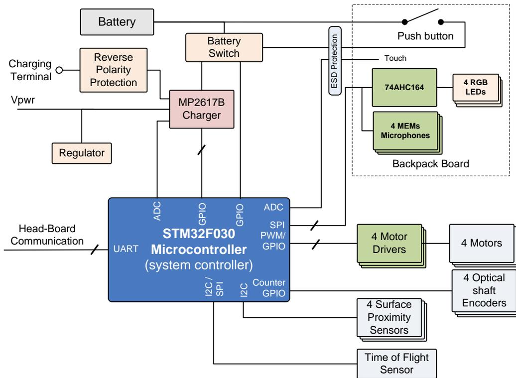
Figure 10: Body-board block diagram
