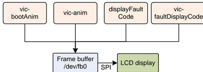
**Figure 31:** The LCD architecture
