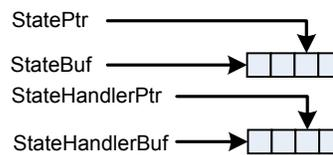
**Figure 10:** Thread control block
