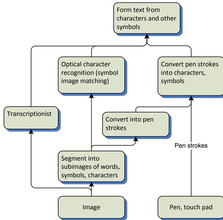
**Figure 4:** Levels of processing in scanning a text
