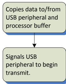
Figure 5: Packet transmission layer of USB
