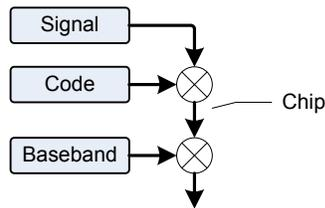
The code increases the transmitted data rate, with a larger bandwidth. It is possible that only a portion of the signal to be received, and all may be briefly not received. The known part of the signal (code) allows the receive to decide what the user data signal was.
