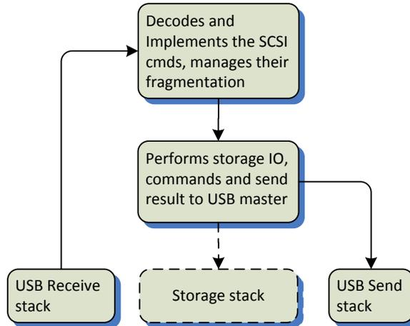
Figure 6: USB stack for mass storage devices
